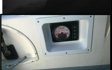
Above - Engine control panel on Sarico with fibreglass housing made using an oven dish as a mould! See write up on page 10. Above and left—
