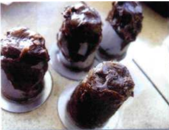
Coatings of diesel bugs blocking tank outlets.
